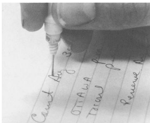
FIG. 2—The ground end of the syringe is placed on top of the ink stroke and gently rotated with firm downward pressure removing a plug paper bearing ink.
