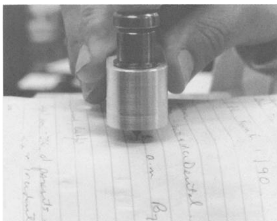
FIG. 5—The punch is best operated from an elevated position which allows easy viewing of the sample area.
