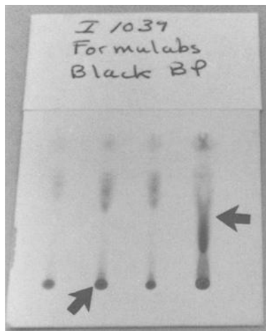
FIG. 11—The deposition of extract onto a TLC plate from an Eppendorf pipetter is difficult to control and can result in spots that are large, diffuse, and generally overloaded. This results in poorly separated dye components with associated tailings (arrow).
